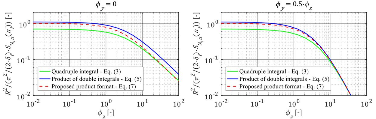
Figure 4. The expression  $R^2 / (\frac{\pi^2}{2\delta_i} S_{N,u}(n_i))$  evaluated for a parabolic mode shape determined by numerical integration of the quadruple integral (Eq. (3)), using the product of two double integrals (Eq. (5)), and using the proposed product format (Eq. (7)). The plots consider  $\phi_y = 0$  (left figure) and  $\phi_y = 0.5 \cdot \phi_z$  (right figure).
