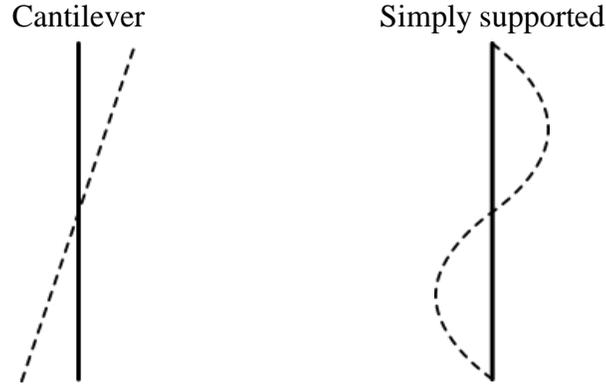
Figure 5. Mode shapes associated with a cantilever and a simply supported structure with three supports.
