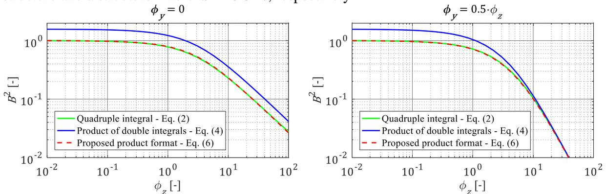
Figure 3. The background response factor  $B^2$  determined by numerical integration of the quadruple integral (Eq. (2)), using the product of two double integrals (Eq. (4)), and using the proposed product format (Eq. (6)). The plots consider  $\phi_y = 0$  (left figure) and  $\phi_y = 0.5 \cdot \phi_z$  (right figure).
