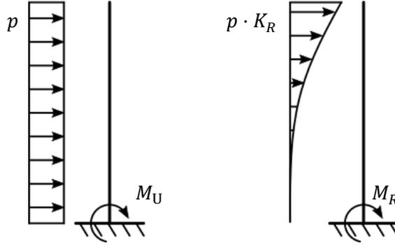
Figure 2. For mode shapes of constant sign, the load distribution factor  $K_R$  is the scaling of a load distribution proportional to the mode shape resulting in a response identical to that of a uniform load distribution, i.e.  $M_U = M_R$ .
