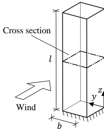
Figure 1. Example of model structure of width  $b$  and height  $l$ .
